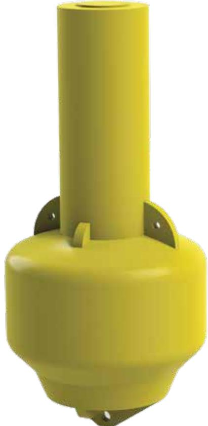
Tritonbuoys has developed a diverse selection of navigation buoys that adhere to rigorous quality standards and boast a proven track record of reliability. Each buoy is crafted from premium UV-stabilized virgin polyethylene and filled with closed-cell polyurethane to prevent water ingress if the outer layer is damaged. This design ensures exceptional performance and long-lasting durability.
